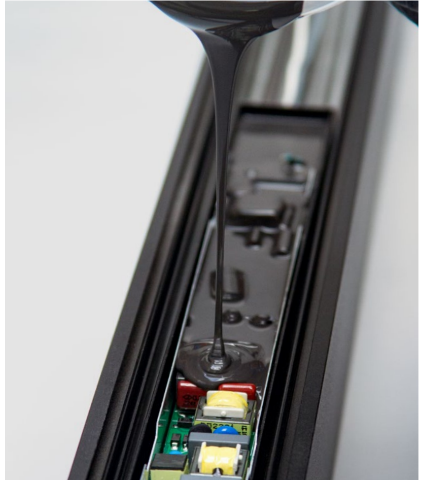
An anthracite grey two component silicone elastomer is used to protect all electronic components, by filling the custom designed driver housing.
