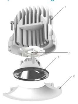
When unscrewing both screws (1) (DIN 912 M3x12), the frontplate (2) comes appart. This frontplate keeps the reflector (3) and the LED array (4) in place. Be very careful when unplugging the LED array (4) from the electrical connector (5)
